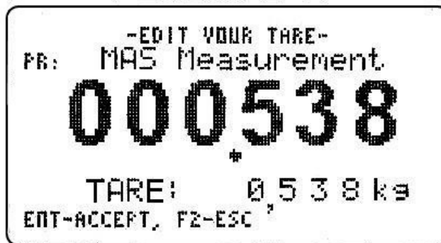
Figure 11: Edit Tare Value screen. This screen is displayed after pressing the <F2> key following the product selection from Figure 10.
